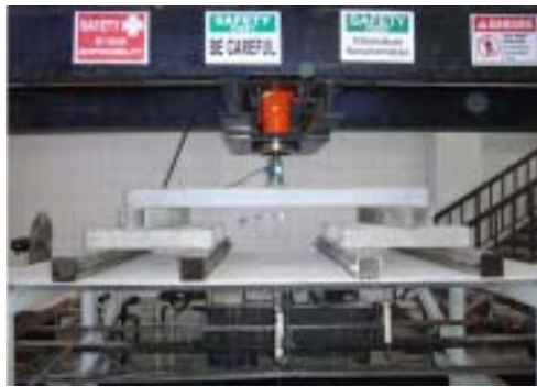
Fig. 4. Image of test set-up details and testing of a PSSDB floor panel
